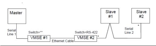
\* Termination is required across RD or RX terminals at these locations if the serial line is greater than 6 feet (2 meters) long
