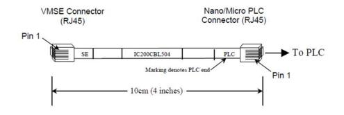
Figure 24 Wiring Diagram for IC200CBL504
